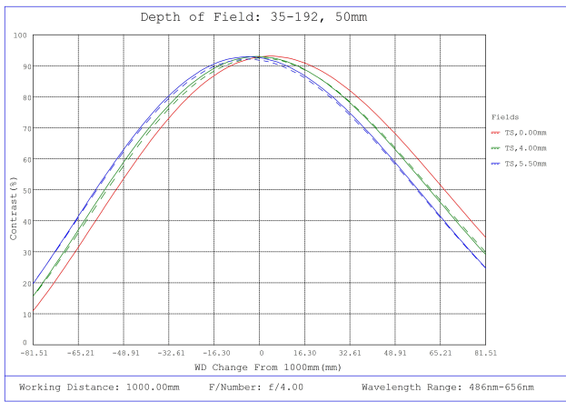
#35-192, 50mm, f/4.0 Cr Series Fixed Focal Length Lens, Depth of Field Plot, 1000mm Working Distance, f4
