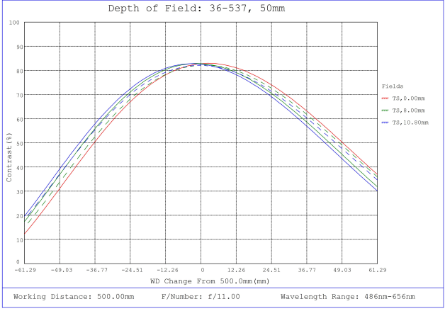
#36-537, 50mm f/11, HPr Series Fixed Focal Length Lens, Depth of Field Plot, 500mm Working Distance, f11
