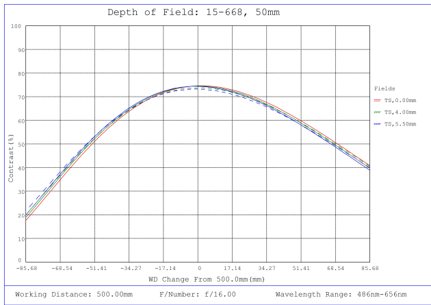
#15-668, 50mm, f/16 Sealed Cw Series Fixed Focal Length Lens, Depth of Field Plot, 500mm Working Distance, f16
