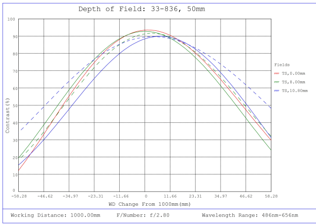
#33-836, 50mm f/2.8, HPI Series Fixed Focal Length Lens, Depth of Field Plot, 1000mm Working Distance, f2.8
