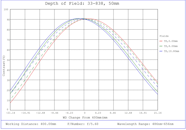
#33-838, 50mm f/5.6, HPi Series Fixed Focal Length Lens, Depth of Field Plot, 400mm Working Distance, f5.6
