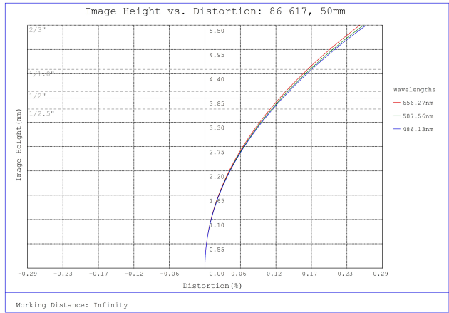
#86-617, 50mm, f/5.6 Ci Series Fixed Focal Length Lens, Distortion Plot
