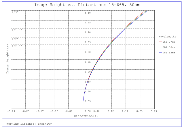
#15-665, 50mm, f/5.6 Sealed Cw Series Fixed Focal Length Lens, Distortion Plot
