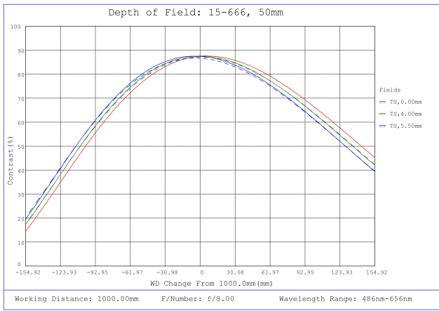
#15-666, 50mm, f/8.0 Sealed Cw Series Fixed Focal Length Lens, Depth of Field Plot, 1000mm Working Distance, f8
