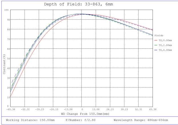
#33-863, 6mm, f/2.8 UCi Series Fixed Focal Length Lens, Depth of Field Plot, 150mm Working Distance, f2.8
