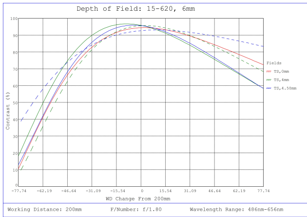
#15-620, 6mm, f/1.8 Cw Series Fixed Focal Length Lens, Depth of Field Plot, 200mm Working Distance, f1.8
