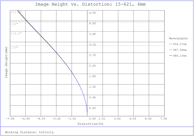
#15-621, 6mm, f/2.8 Cw Series Fixed Focal Length Lens, Distortion Plot
