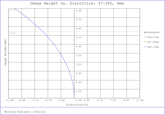
#37-382, 6mm FL f/2.5, Rugged Blue Series M12 Lens, Distortion Plot
