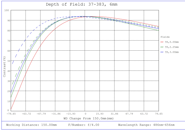
#37-383, 6mm FL f/4.0, Rugged Blue Series M12 Lens, Depth of Field Plot, 150mm Working Distance, f4
