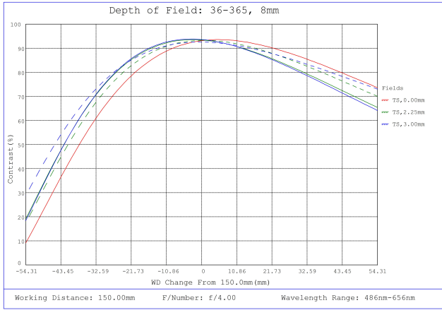
#36-365, 8.0mm FL f/4 Rugged Blue Series M12 Lens, Depth of Field Plot, 150mm Working Distance, f4
