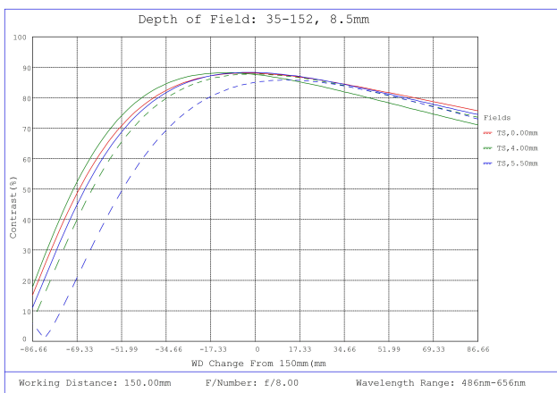
#35-152, 8.5mm, f/8.0, 75mm-∞ Primary WD, HRr Series Fixed Focal Length Lens, Depth of Field Plot, 150mm Working Distance, f8
