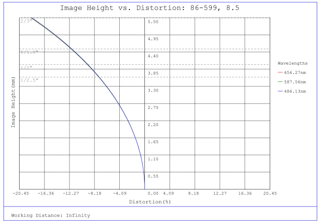
#86-599, 8.5mm, f/1.3 Ci Series Fixed Focal Length Lens, Distortion Plot
