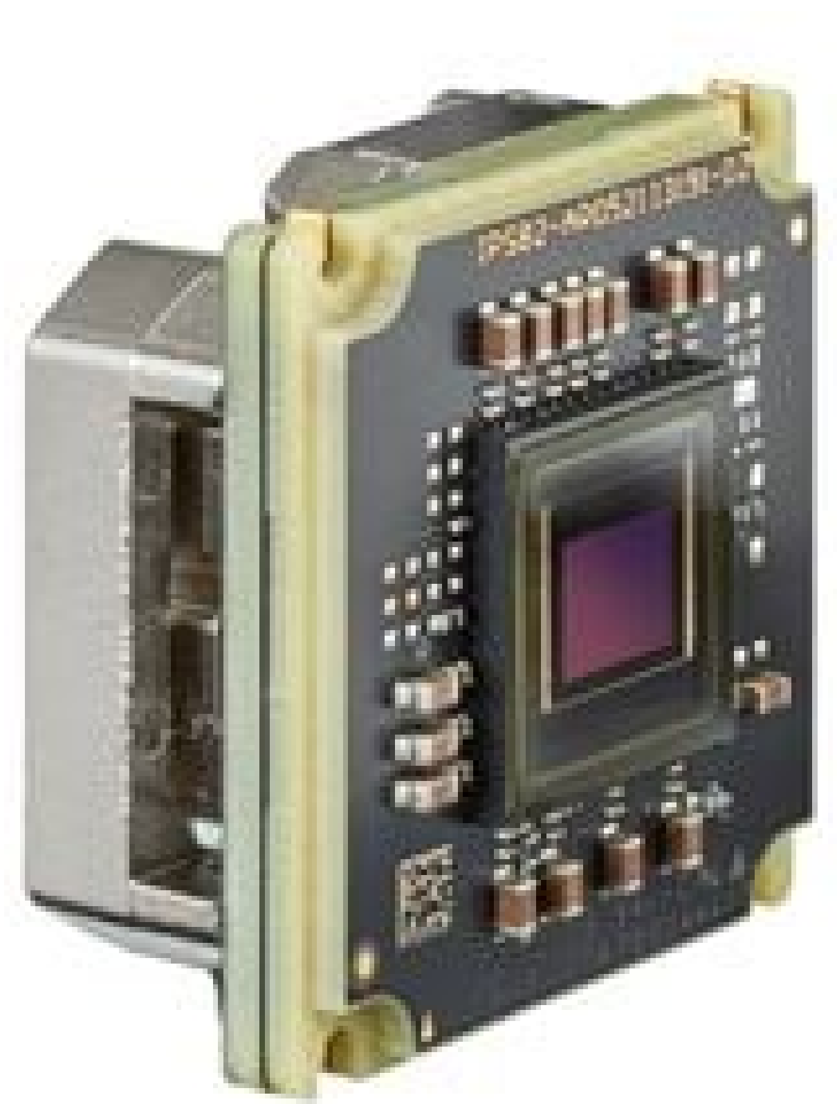
Allied Vision Alvium Camera, Board Level (Front)
