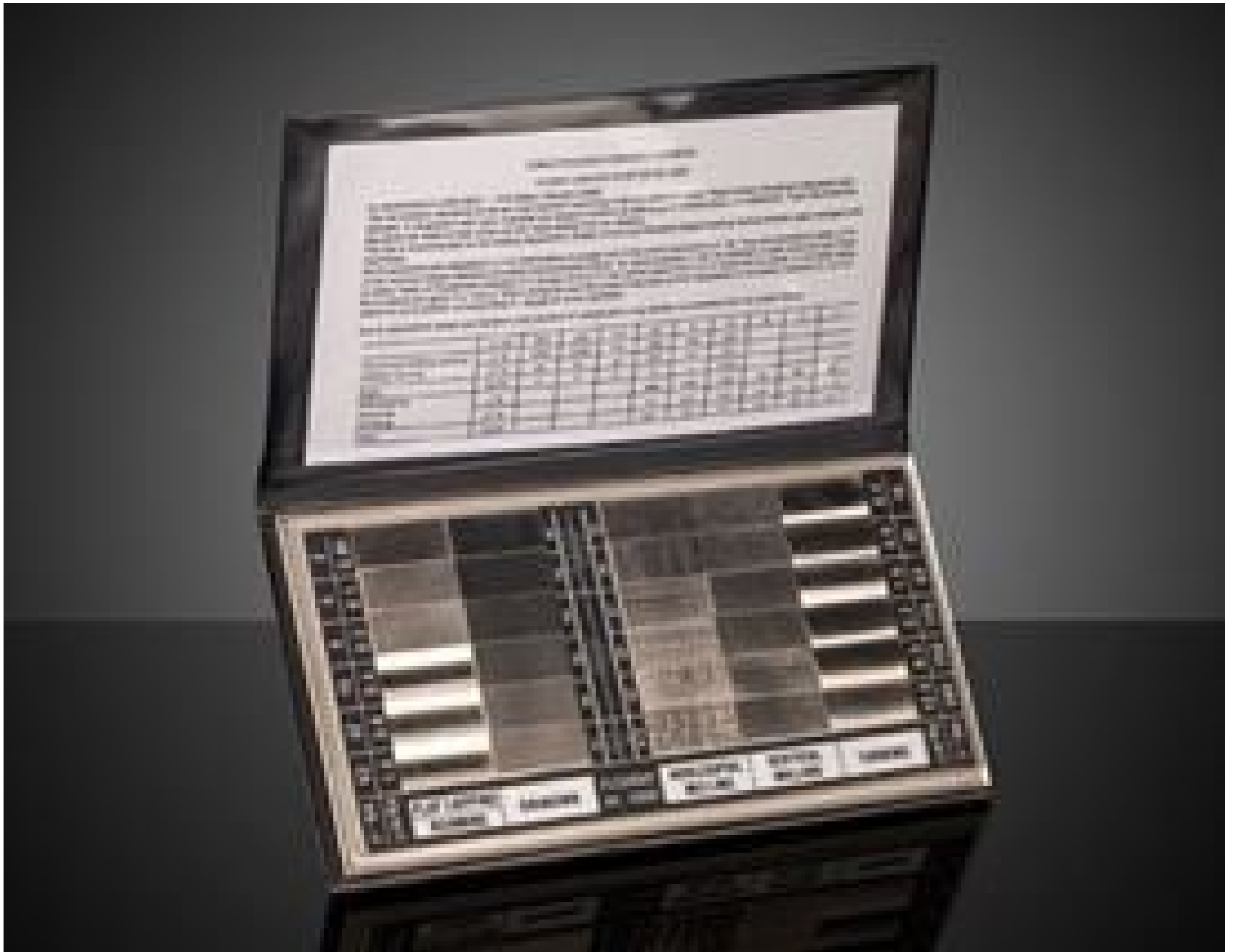
Surface Roughness Standard
