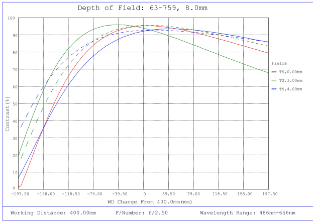
#63-759, f/2.5, Visible, 8.0mm HEO Series M12 Lens, Depth of Field Plot, 400mm Working Distance, f2.5
