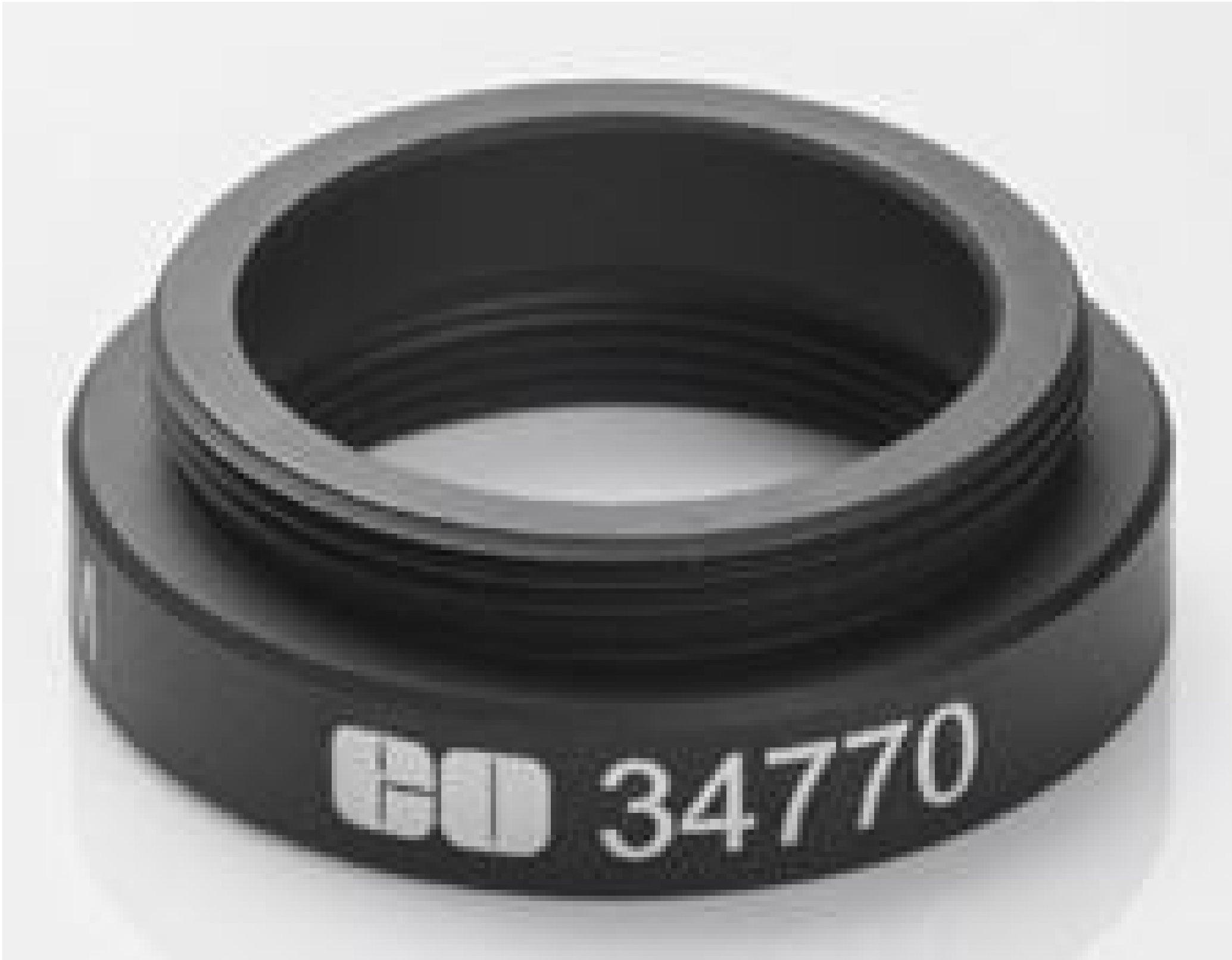
Female M22 x 0.75 to Male C-Mount Adapter, #34-770
