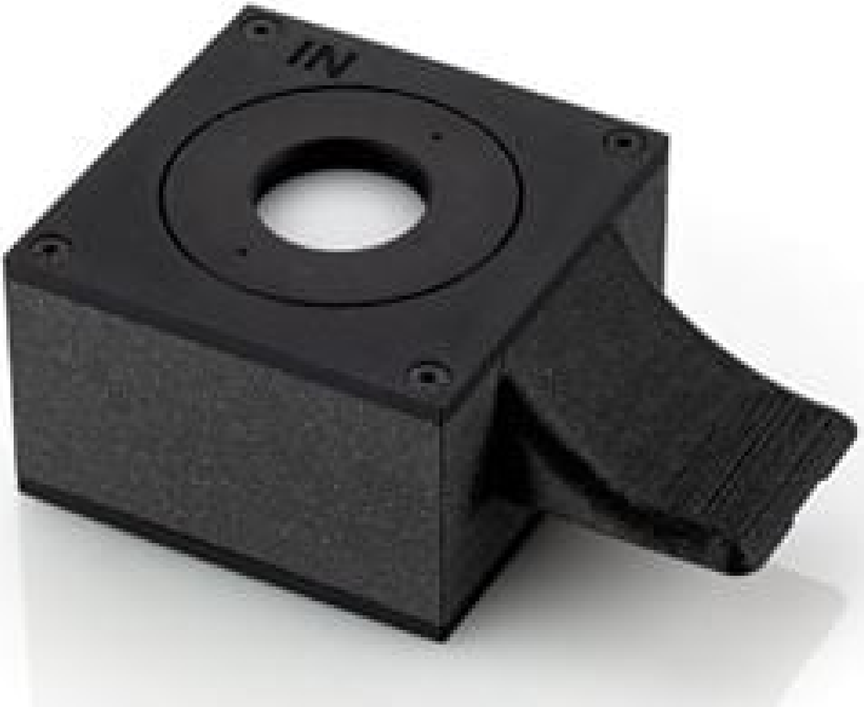
fNIRS Standard Phantom - IEC 80601-2-71
