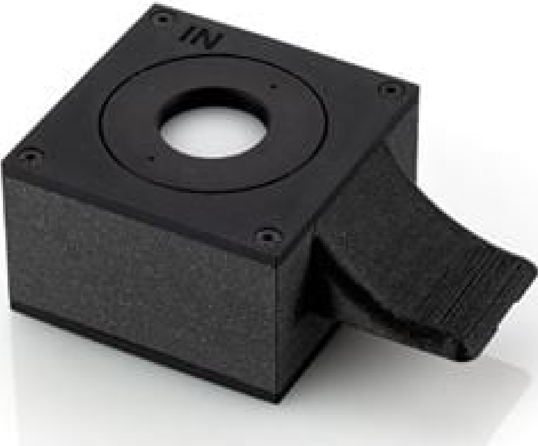
fNIRS Standard Phantom - IEC 80601-2-71
