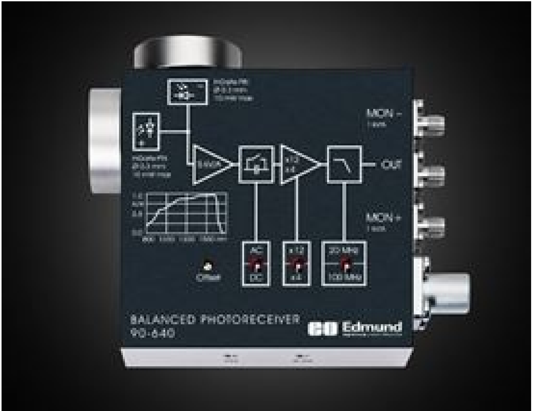
#90-640 InGaAs Free-Space Balanced Photoreceiver, 800-1700nm
