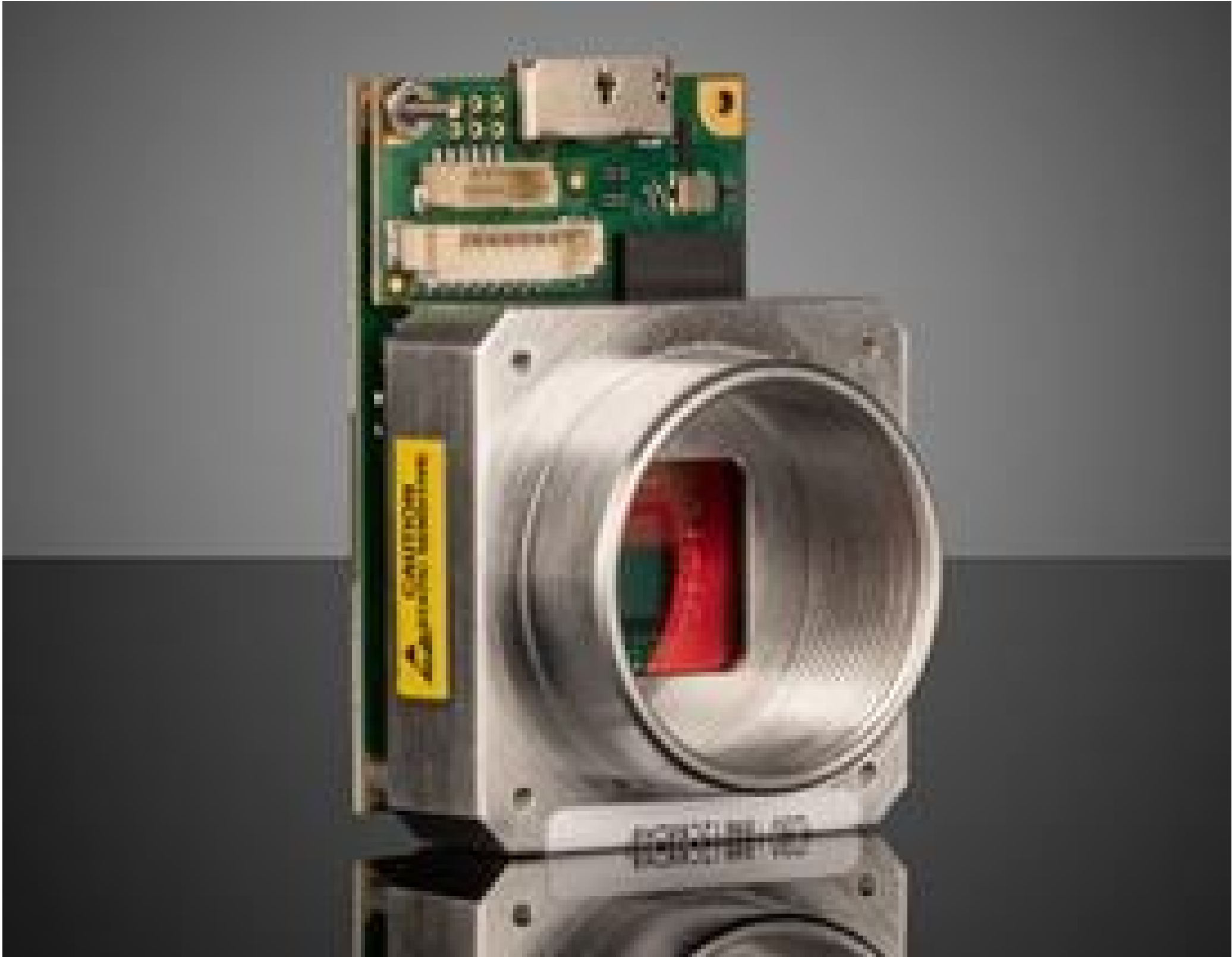
Pixelink® USB 3.0 Cameras (Board Level)
